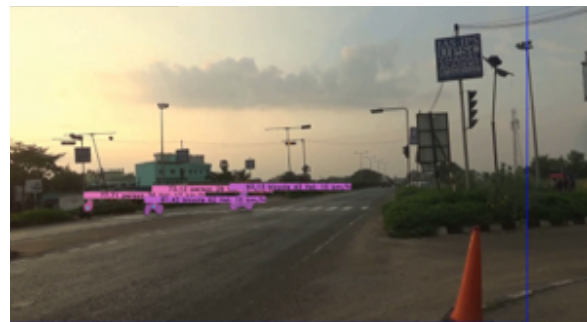
Fig. 8b: Detected vehicles in a frame of video 00130
